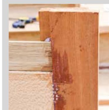
**1** The corner support was created from two blocks of mahogany, cut to the thickness of the bulkhead.
