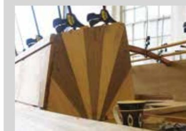
**5** This bulkhead has a split, but it'll be easily fixed with epoxy mixed with a little sawdust of the same wood.
