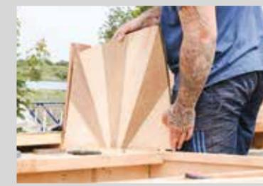
**4** The bulkhead with its decorative veneer of coloured hardwood marquetry is offered up, and when a tight fit is achieved it is epoxied and clamped into place.
