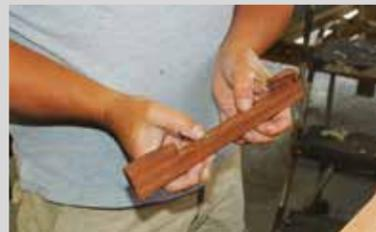
**2** This spar gauge is the secret weapon. Note the two screws set into the timber and how their tips just protrude clear at the bottom.
