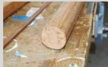
**6** The boom has been planed into equal 16ths, and could be rounded (if required) with 32 sides planed by eye and a final sanding.
