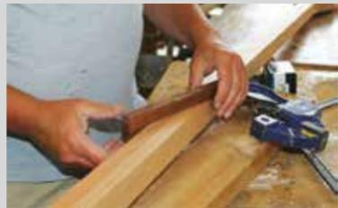
**3** The gauge is laid onto the square box section and run along the full length of all the sides. The ratio stays consistent even if the spar tapers.
