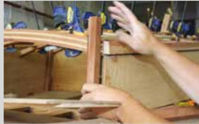
Similar to the rear cabin bulkhead, the forward end starts with a corner post made from two blocks of hardwood glued together with thickened epoxy.
