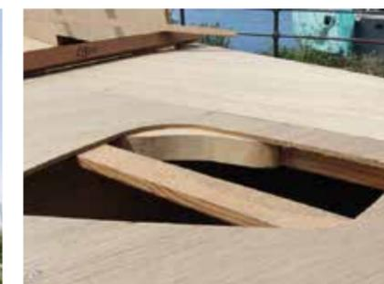
Forward hatch showing lodging knee for sampson post (fore and aft deck frame to be removed)
