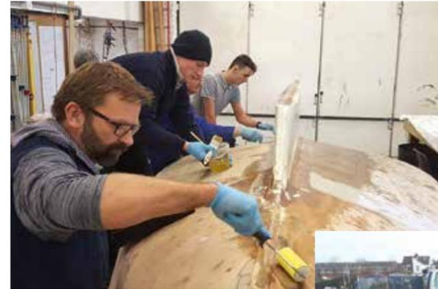
**LEFT** Applying epoxy to the glass cloth sheathing on the hull
