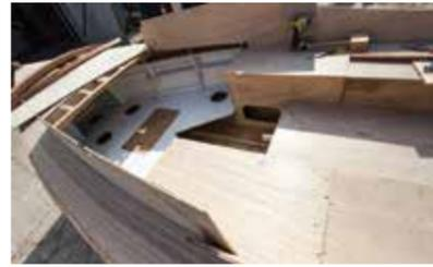
The cabin sides and coaming have here been temporarily screwed into place to check for alignment
