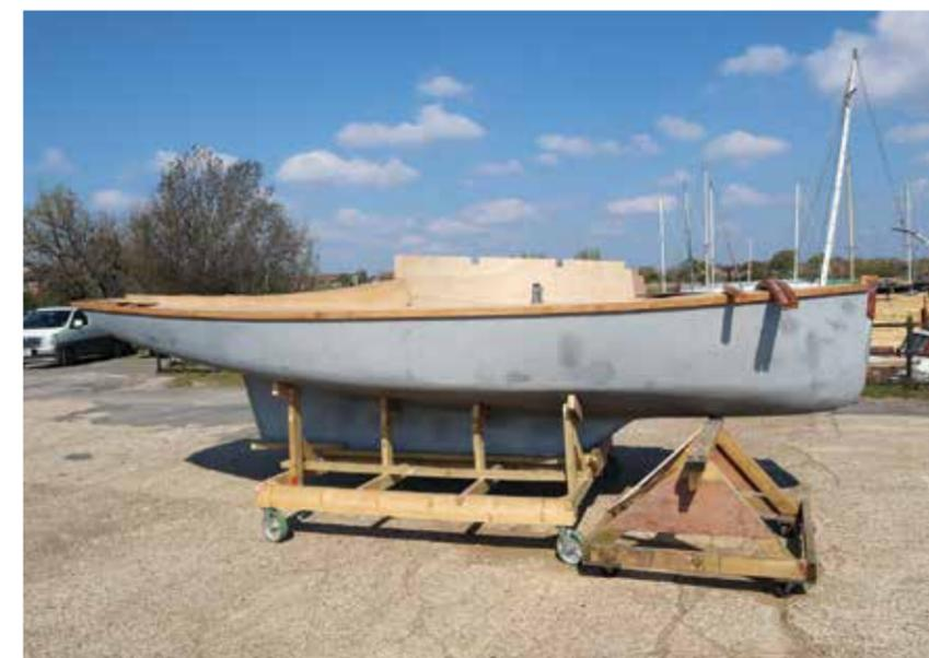
The hull has been returned to its upright position, and now the decks and cabin sides are being added. Note the laminated cross beams, which can be seen lying on the foredeck prior to dry fitting, and the slots they will locate into along the top edge
